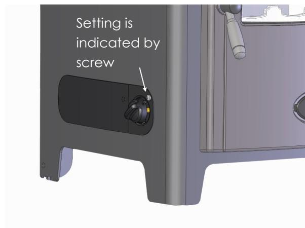
If a lower radiator temperature is required a lower number should be selected. Some experimentation may be necessary to find the setting best suited to your requirements.
