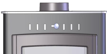
The airwash has an internal sliding plate with slots, housed in a cover plate, and is located above the fire door. Sliding the control knob to the **RIGHT** as far as it will go, achieves the fully open position.
